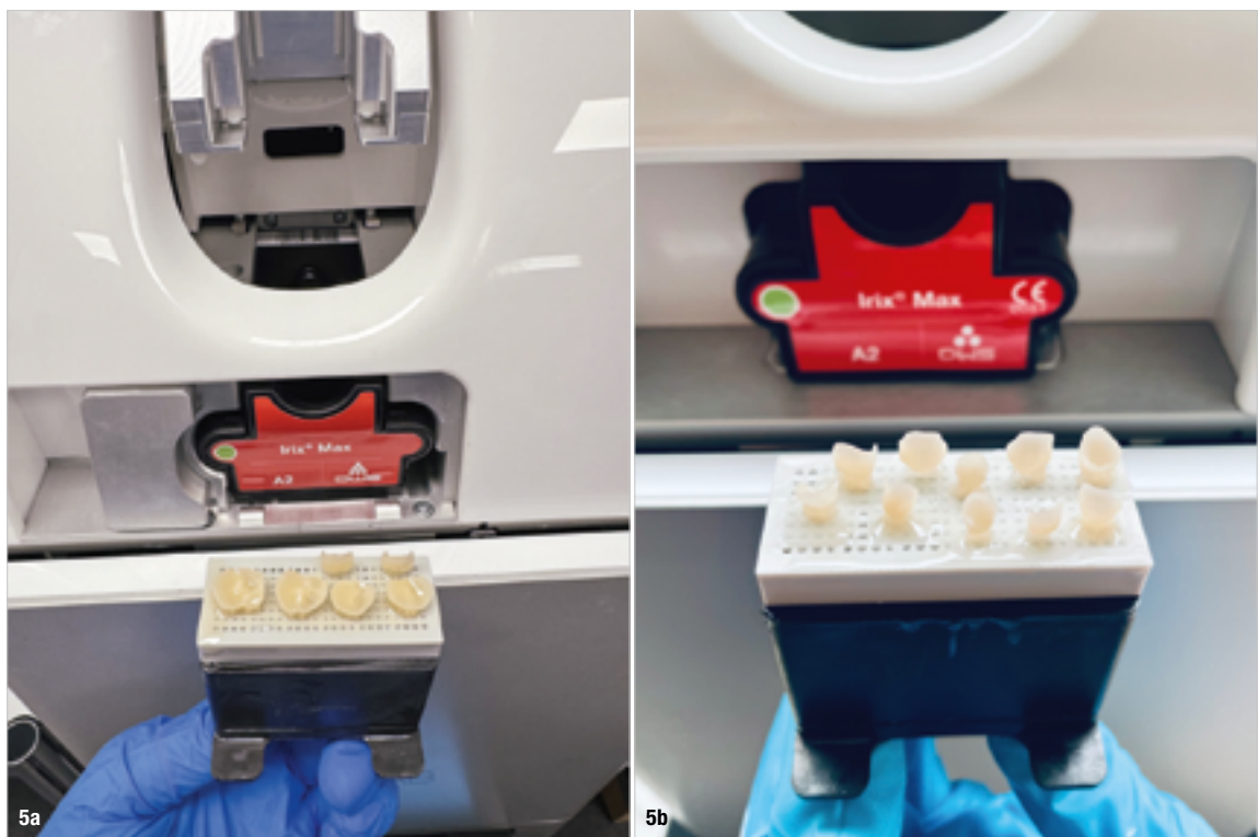
Figs. 5a & b: Restorations produced with the Dfab printer and Irix Max hybrid resin composite.
