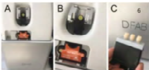
Fig. 6. 3D printing of the prosthetic restoration in hybrid ceramic material (Irix Max®). (A) The DFAB® printer with its printing plate and vat inclusive cartridge in place; (B) Detail of the Irix Max® cartridge with PHOTOSHADE®; (C) the newly fabricated restorations, before removal of the printing plate and washing in alcohol.
