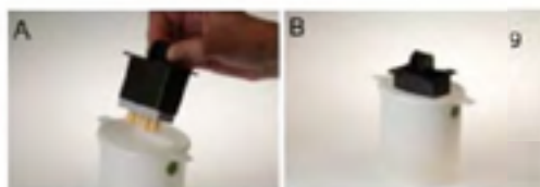
Fig. 9. Washing of restorations in special box with ethyl alcohol. (A) The printing block is inserted inside the box (B) the box is closed and shaken so that resin residues can be washed off the restorations and abutments.
