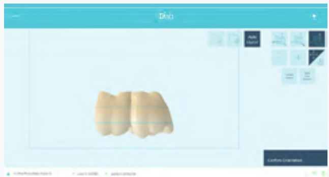
FIG. 5B The Photoshade software automatically orients the virtual restoration for optimal printing and color gradient results.
