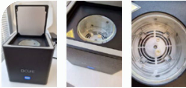
FIG. 7A-C Polymerization in DCURE® (DWS Systems, Italy) oven. (A) View of the DCURE®; (B) the restorations are placed inside the DCURE® unit; (C) top view of the restorations after the curing process. The whole process takes only 5-8 minutes.
