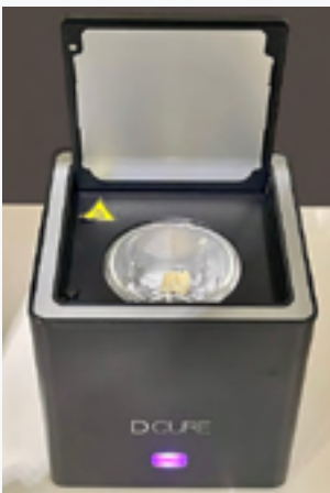
FIG. 8A, B (A) The Dcure UV and heat post-polymerization unit containing the treated restoration. (B) Occlusal view of the post-polymerized restoration.
