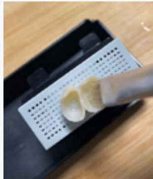
FIG. 7A-D (A) Washing with 95% ethanol using a shaker for one to two minutes. (B) Scrubbing the intaglio surfaces with a brush wetted in 95% ethanol helps remove liquid composite residue. (C) Once the restoration has been separated from the platform, its occlusal surfaces are also scrubbed to remove any liquid composite traces. (D) An intaglio view of the restoration after washing and drying, ready for post-polymerization.
