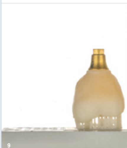
Fig. 9: Dfab-printed crown, still on the platform, after washing with 95% ethanol and drying. Fig. 10: Dcure post-polymerisation unit. Figs. 11 & 12: Finished crown cemented to the Ti-base with a dual-polymerising resin cement.
