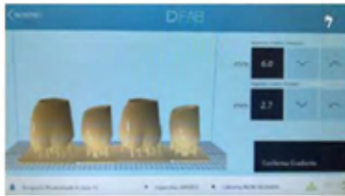
Fig. 7. Screenshot of DFAB ® Photoshade software for setting color gradients.
