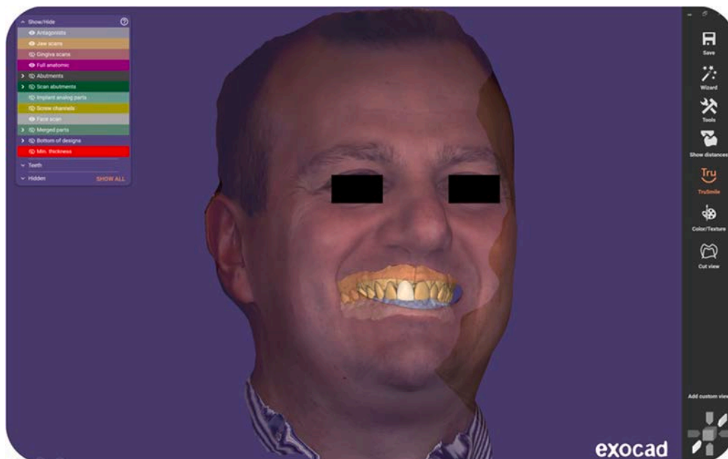
Fig. 7. CAD modelling (Galway®, Exocad, Darmstadt, Germany) of the crown in relation to the patient’s face, acquired with a face scanner (RAYface®, Ray, Hwaseong, South Korea).
